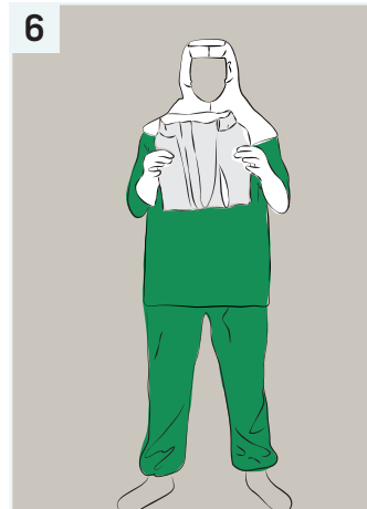
6 Touching the inner surface, take the coverall and hold outwards, allowing the coverall legs to partially unfold.
